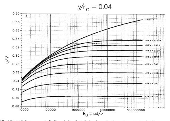
Fig. 1. Chart for predicting mean velocity from single-point velocity observation for turbulent flow in circular pipes;  $y/r_0 = 0.04$ .
