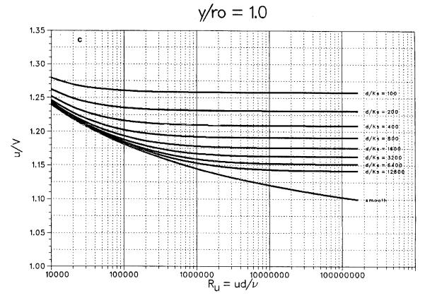
Fig. 3. Chart for predicting mean velocity from single-point velocity observation for turbulent flow in circular pipes;  $y/r_0 = 1.0$ .
