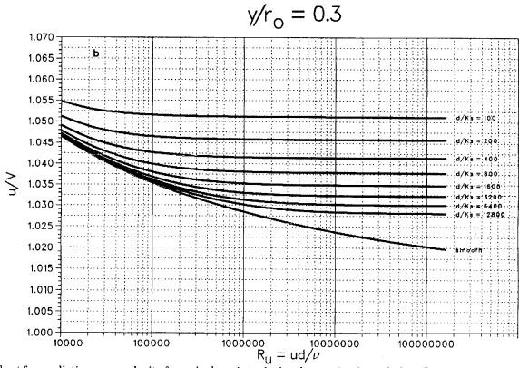
Fig. 2. Chart for predicting mean velocity from single-point velocity observation for turbulent flow in circular pipes;  $y/r_0 = 0.3$ .
