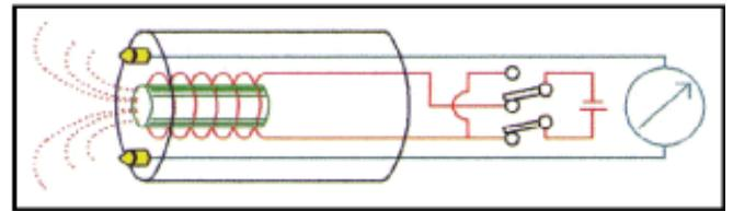
Magnum IC houses a full featured digital transmitter inside the sensor housing itself. All features of the basic flowmeter, plus a number of possible optional additions, including pressure and temperature sensing, as well as data-logging, are enclosed within the compact submersible package.
