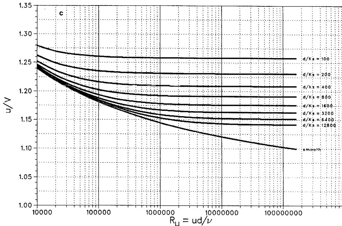
Fig. 3. Chart for predicting mean velocity from single-point velocity observation for turbulent flow in circular pipes;  $y/r_0 = 1.0$ .
