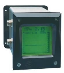
Magnum is an entirely digital instrumet. All internal functions of the flowmeter are controlled by software. Setup and configuration for applications are handled by the Magio 3.0 software interface, which runs on any Windows based PCs. Setup can be done in the field on a laptop or in the office at a desktop PC.
